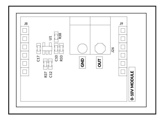
To use 0-10V from 0-10V Module or J26 connector, place a jumper as shown on the board.
