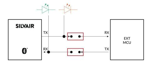
RX/TX signals are also connected to the J25 connector for debugging purposes.
