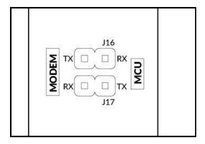
Additionally, there are two LEDs on the Modem side which are connected to RX (green LED) and TX (amber LED).
